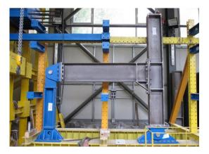
Particular results are represented by the selection of members (beams & columns) from the analyzed frames, and the development of a design procedure for bolted beam-to-column haunched connections. The pre-test numerical simulations lead to some adjustments of the joint design procedure and joint configurations. As a result, the joint configurations were established and the experimental test set-up was designed. Finally, the shop drawings for joint specimen and test set-up were completed.
